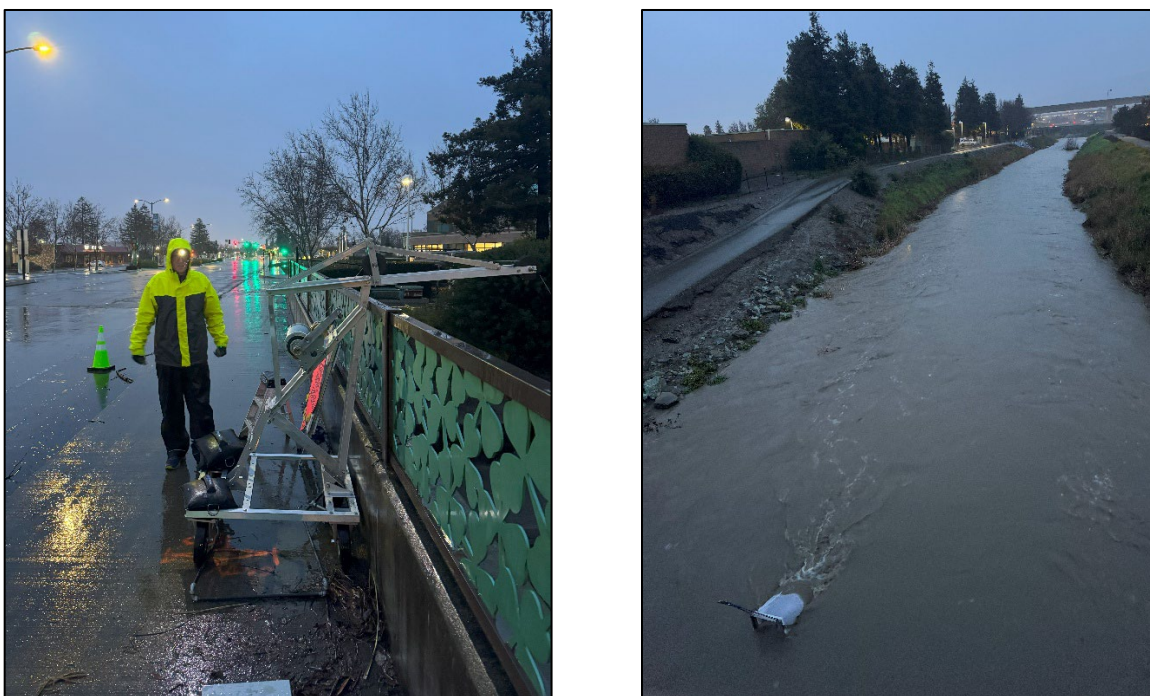
Figure 2 Monitoring equipment modified box trawl (right) trawl deployed from a bridge crane (left)
