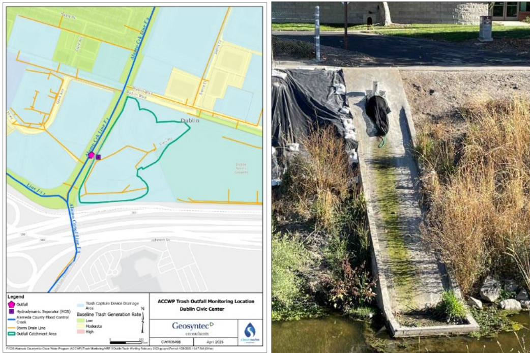
Figure AC-4. AC-CVIC outfall with the NetTech monitoring device (east bank of Alamo Canal, Dublin)
