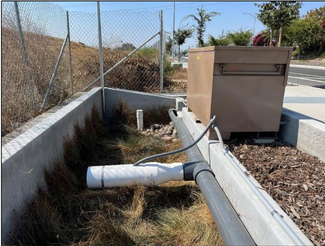
Figure 3.3 Influent collection device, weir, and ISCO enclosure at TCM4 at the Top Golf Public Green Streets Project in San José, CA.
