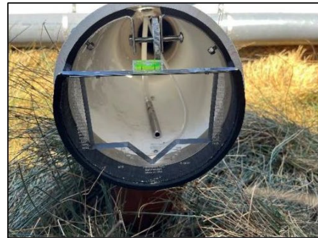
Figure 3.3 Influent collection device, weir, and ISCO enclosure at TCM4 at the Top Golf Public Green Streets Project in San José, CA.
