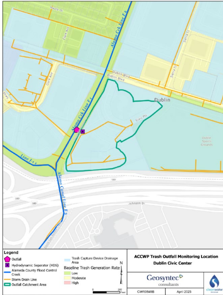
Figure AC-2. Trash monitoring catchment area at Civic Center in the City of Dublin.
