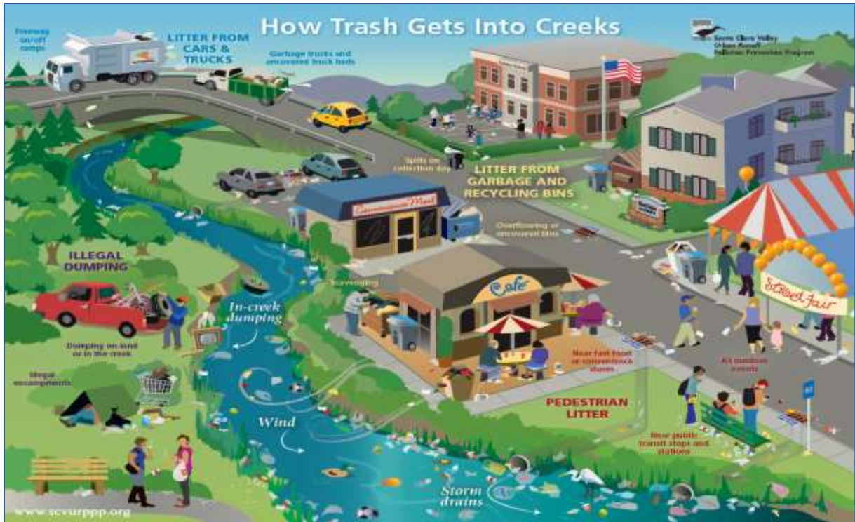
Figure 2. Potential trash sources and transport pathways, including stormwater, to surface waters (SCVURPPP 2010)
