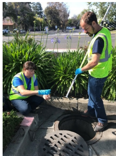
Sediment sample collection with pole in maintenance hole
