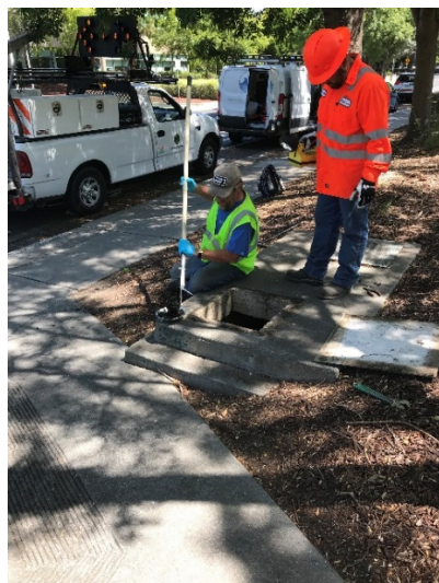
Sediment sample collection with pole in vault
