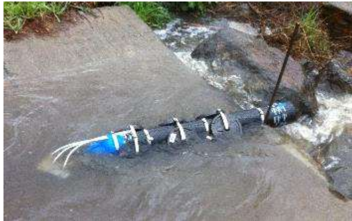
Figure 2. Sampling equipment used in the field. (a) Painters pole, Teflon tubing and an ISCO used as a slave pump; alternatively a Teflon bottle is attached to the end of a painters pole (DH84) and used for sample water collection as opposed to using an ISCO as a pump (b) Hamlin suspended sediment sampler; and (c) the Walling tube suspended sediment sampler.
