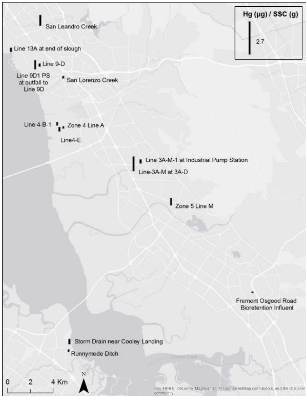
Figure 9c. Distribution of sites and particle ratios of total mercury (HgT) in stormwater samples collected to date in southern Alameda and San Mateo counties.
