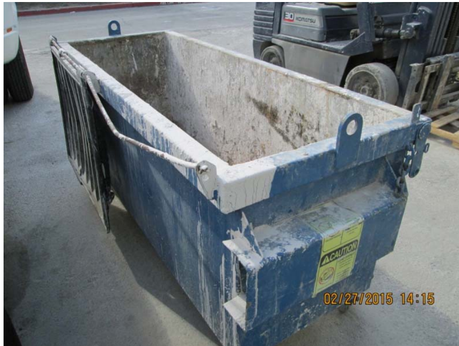
Dumpster missing a lid
