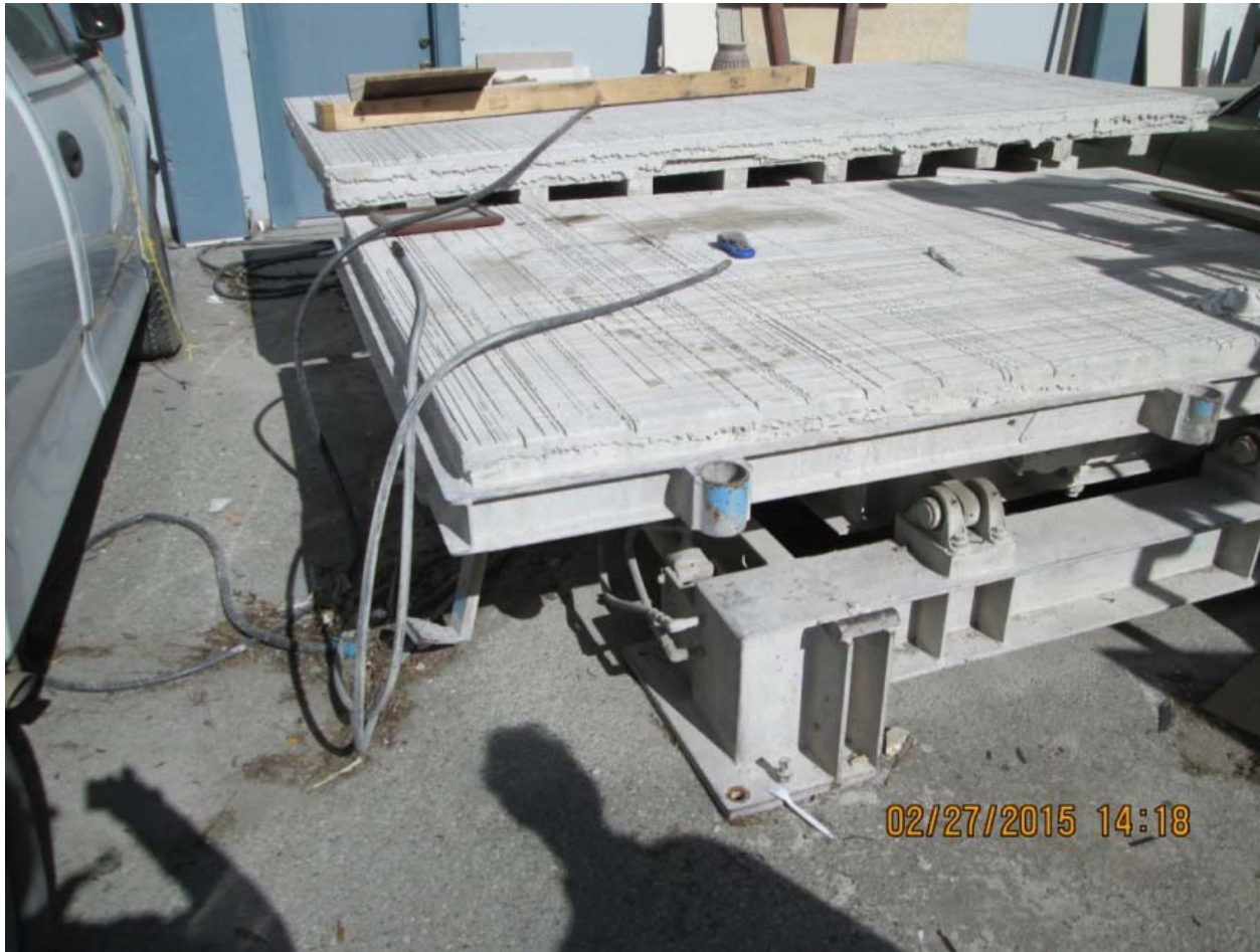
Stone cutting table stored outdoors with cutting dust on it
