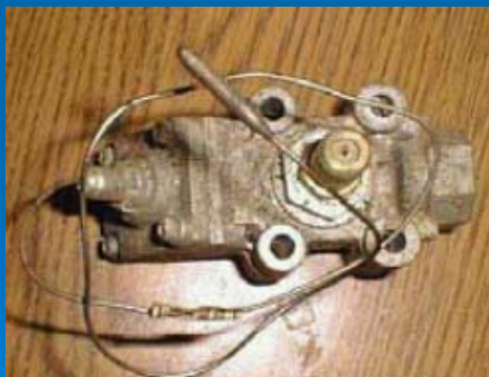
Flame Sensor from Gas Range
