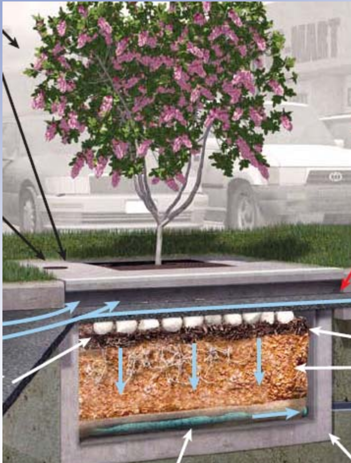
Example of a Manufactured Tree Well Filter
